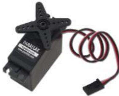
Figure 8, Parallax Standard Servo
